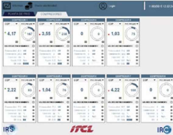
Figure 5.16 - IRS, industrial refrigeration supervision
